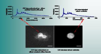
SERS images and spectrum of cresyl violet dye adsorbed onto 75  $\mu m$  silver coated-silica beads (left) and CV-labeled silver colloidal particles (right). The images were acquired with the AOTF device set at a SERS intensity signal of 596 cm-1 using a 632.8 nm HeNe laser for excitation. Scale bar, 75  $\mu m$ .
