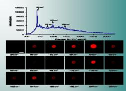
SERS spectrum and images of cresyl violet-labeled silver colloidal particles collected at various surface-enhanced Raman shifts. The images were acquired by scanning the AOTF over the entire spectrum using a 632.8 nm HeNe laser for excitation. Scale bar, 75 µm.
