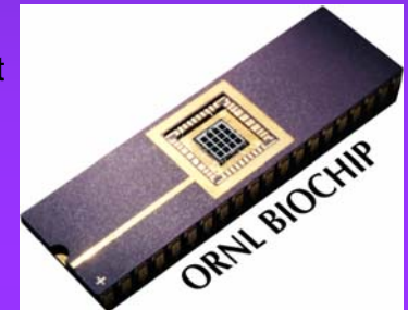
Figure 3: Photograph of the integrated circuit detection system of the Biochip
